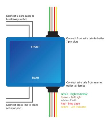
Wiring diagram above applies to Credo™ pre-assembled Brake Controller with hydraulic brakes only.
