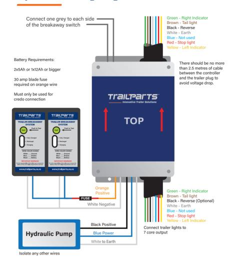
All unused wires on pump and Credo must be isolated.
