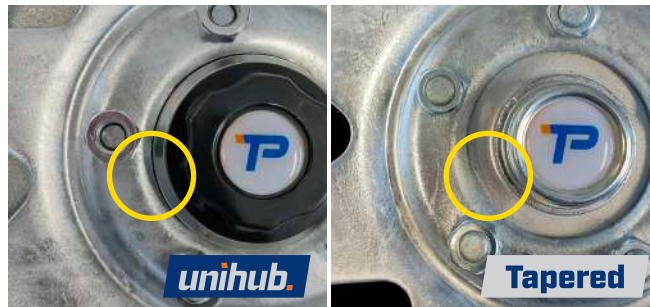
Clearance fit - No gap
